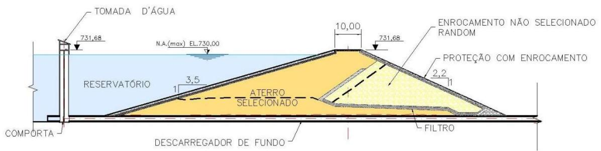
**Figura 5.2-5 – Tomada D'Água - Corte**
